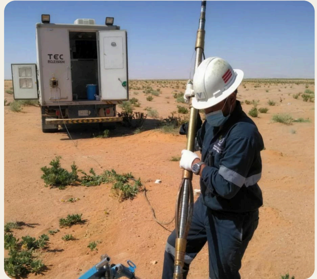
Wireline logging at a water well
