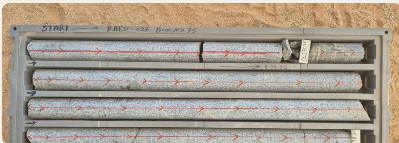
Drill core laid out in its tray for logging and sampling
